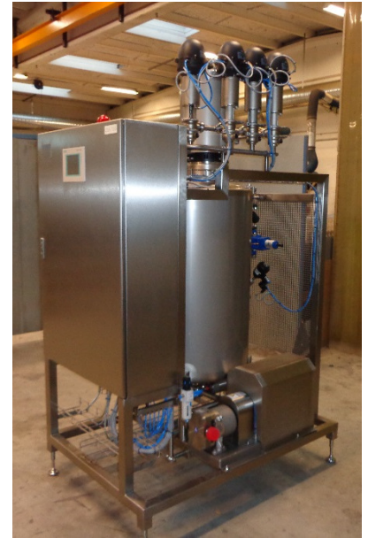
Complete sludge cooker. This is made for a dairy to handle the sludge from their separator.
