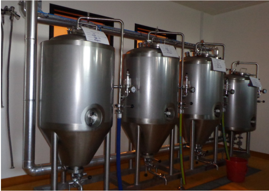
Fermenting tanks and a pressurised balance tank for small-scale beer-brewing.
